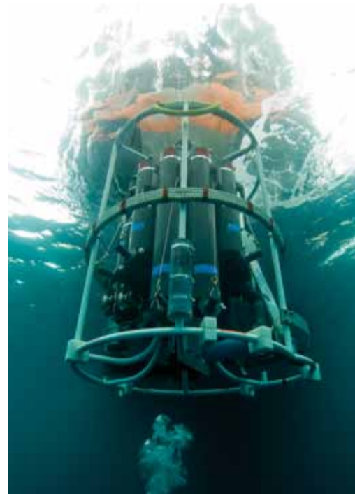
The Rosette is a seawater sampling device. © J.Girardot/Fonds Tara
