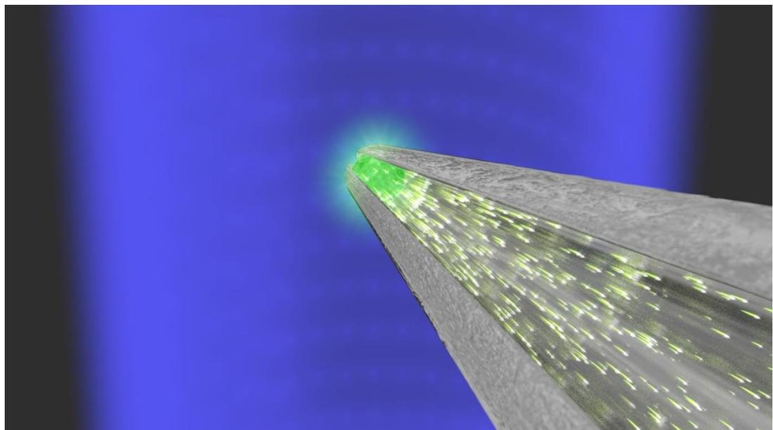
*Optical antenna coupled to a scintillation cluster attached to the end of an optical fiber. The blue beam represents X-ray radiation; the intense, bright green sphere is the scintillation cluster; and the sparks within the body of the optical antenna are the photons emitted by the scintillators after absorbing X-rays. The optical antenna strongly directs this emitted light toward a very narrow single-mode optical fiber.*
