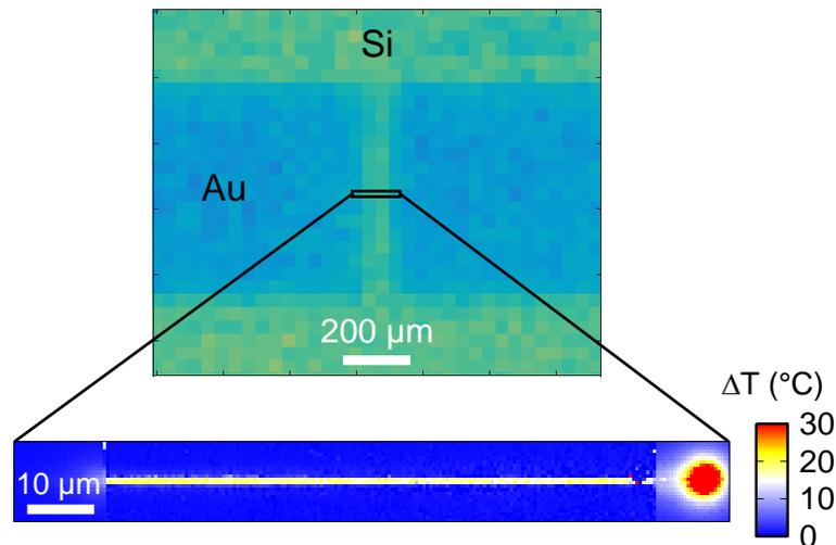
Temperature map of a gold nanowire on a silicon substrate, Joule-heated by the application of an electrical current of 7 mA, obtained through infrared thermography (top) and a spin-crossover surface thermometer (bottom). While heating remains undetectable in infrared due to low thermal and spatial resolution, temperature distribution is well resolved using an SCO-based thermometer, which reveals a “hot spot” resulting from a malfunction of the component.
