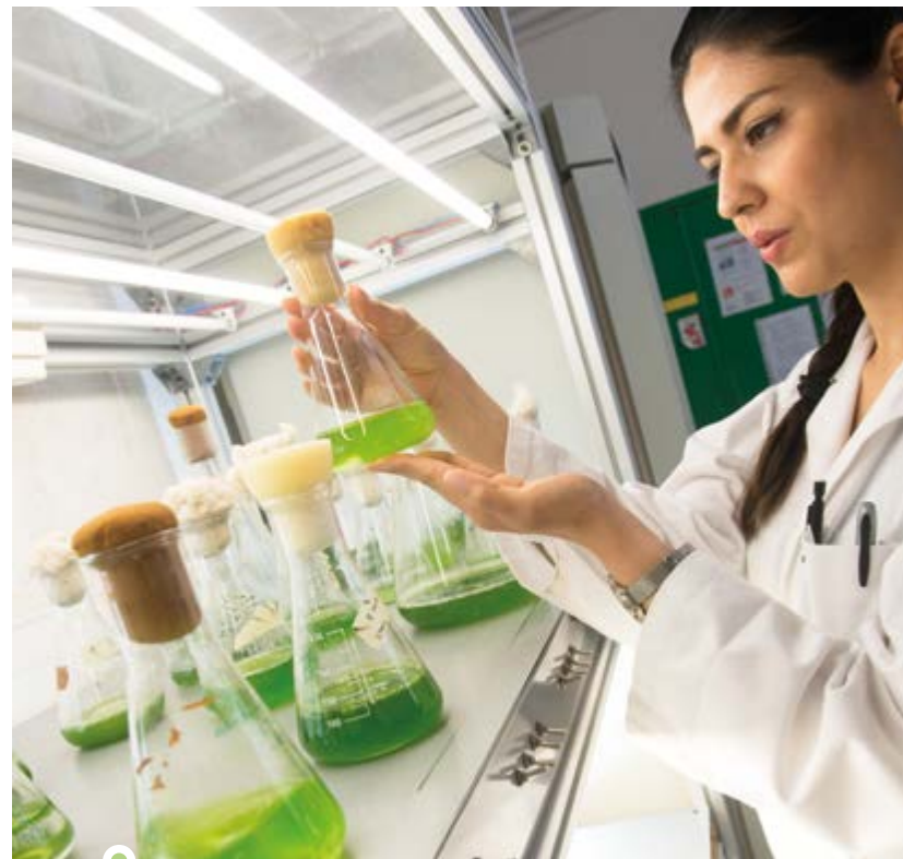
Cultures of Parachlorella kessleri and Chlorella vulgaris microalgae arranged on a shaking tray to obtain starters for cultures in larger bioreactors.
