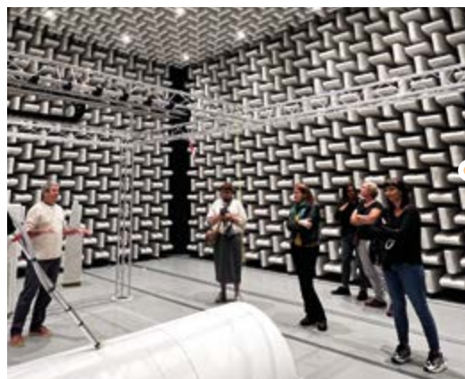
A visit to an anechoic chamber at the Laboratory of Mechanics and Acoustics in Marseille. This exceptional environment features the (almost total) absence of reverberation which creates a unique sensation of sound insulation that is ideal for high-precision acoustic testing. © CNRS / Haguenauer
