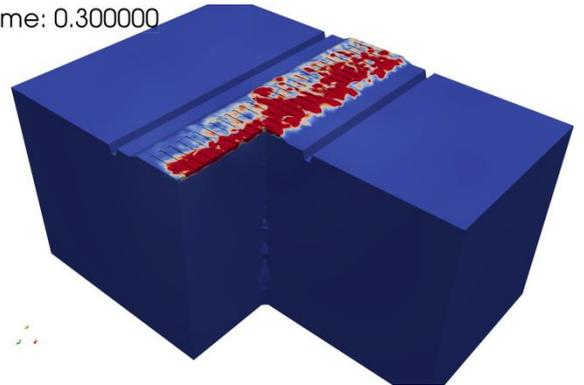
*Amplitude of the displacement field after a train passes on the track. The left-hand figure corresponds to a simulation with homogeneous ballast and the right-hand image to a simulation with heterogeneous ballast. © Lucio de Abreu Corrêa, Laboratoire de Mécanique des Sols, Structures et Matériaux (CNRS/CentraleSupélec)*
