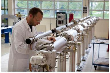
Assembly of cryogenic helium distribution system for series of cavities along XFEL  $\ensuremath{\mathbb{C}}$  Dumas / CEA
