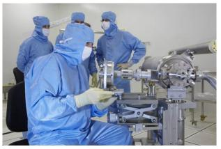
Clean-room assembly of accelerator cavities © Dumas / CEA
