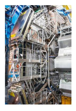
Figure 3: ©Cyril Fresillon/LHC/CNRS Photothèque- Atlas, the largest particle detector ever built for particle physics (46m long and 25m high), opened during a stoppage. Designed to help us understand our Universe and how it evolved, it detects elementary particles produced during proton-proton collisions.
