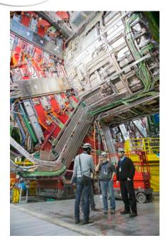
Figure 2: ©Cyril Fresillon/LHC/CNRS Photothèque-Technician doing maintenance on the CMS (Compact muon solenoid), a large detector in the Large Hadron Collider (LHC), during a long technical stoppage (2013-2015).
