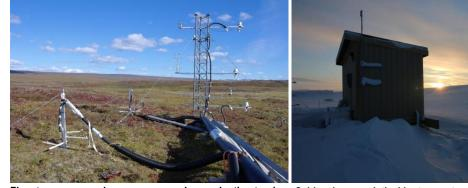
Flux tower measuring mercury exchange in the tundra at Toolik Field Station in Alaska
