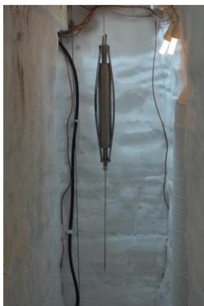
Temperature probe developed at the Institute of Environmental Geosciences (OSUG, CNRS / IRD / UGA / Grenoble INP) to collect data from the EPICA borehole at Concordia.
