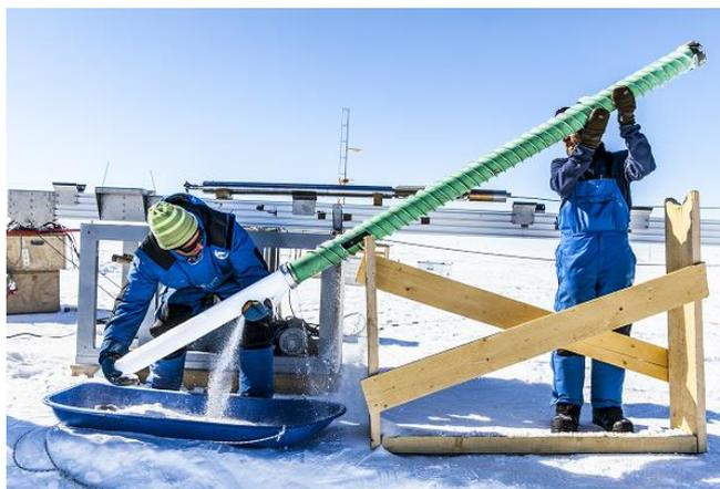
Testing the prototype of the Mini-Subglacior experimental probe.
