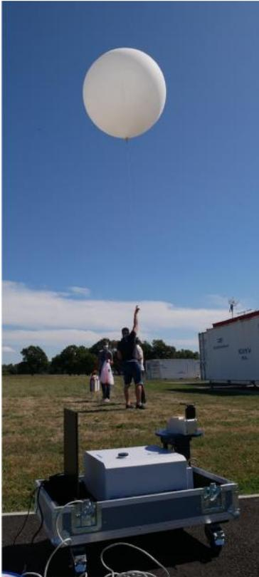
**Release of a weather balloon carrying an AirCore sampler** from CNES's Aire-sur-l'Adour site in 2020. The AirCore sampler collects a sample of air which is subsequently analysed. In the foreground: an EM27/SUN spectrometer.
