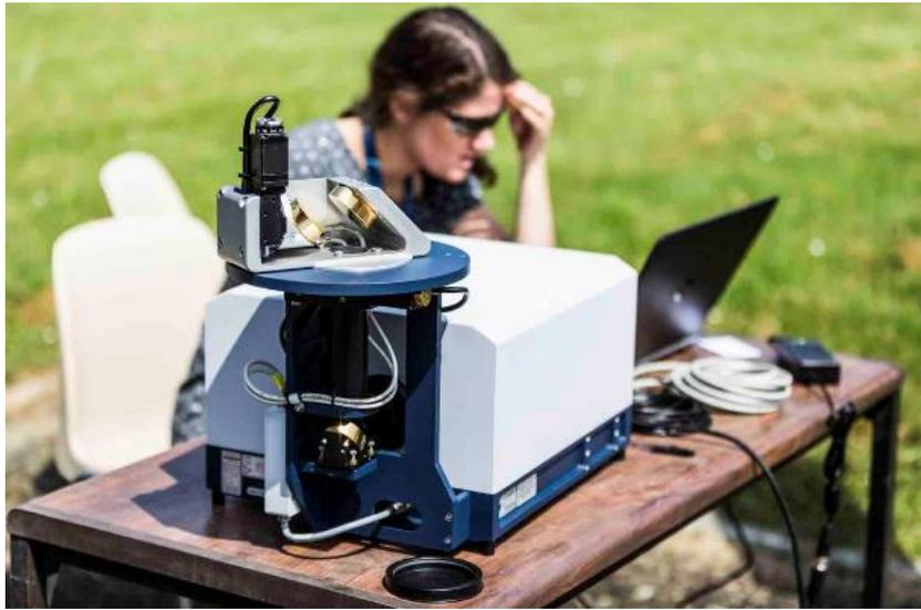
**Deploying an EM27/SUN spectrometer at the Aire sur l'Adour site on May 24, 2018.** This instrument measures concentrations of greenhouse gases in an entire column of atmosphere.
