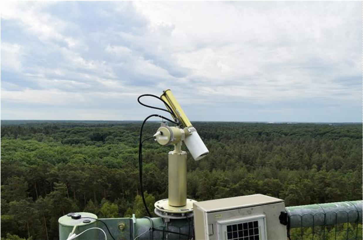
**Photometer monitoring aerosol concentrations over Rambouillet forest from the ACROSS observation tower.**
