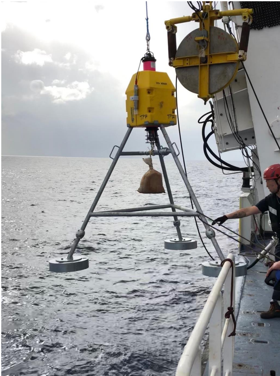
Submersion of seafloor geodetic station (Canopus acoustic beacon) off shore of Catania, aboard ship Pourquoi Pas? , during FocusX1 campaign in October 2020.
