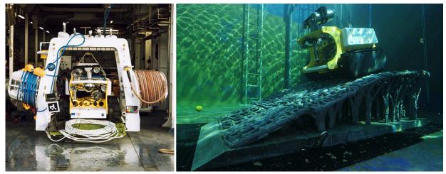
**On the right, Bathybot in its dock aboard the** *Pourquoi Pas?* A 50 m blue cable connects the rover to the dock, which is in turn connected to the scientific junction box, and to the rest of the network via the orange cable.
